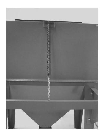
To attach the spring assembly to cabinet, insert <u>spring end</u> through hole in bracket in position at top of cabinet back. To attach opposite end of spring assembly to back rack, tilt cabinet top back and insert Shook into hole in center of horizontal support, bend Shook to secure.
